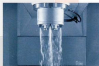
中心出水 需要深孔加工時有利排屑 Center of water Need for deep hole processing good chip removal
